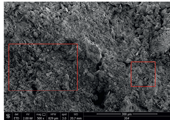
FIGURE 10: SEM of fracture in a saturated state.
