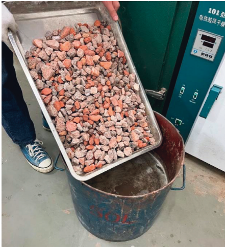
FIGURE 5: PVA solution soaking recycled aggregate.
