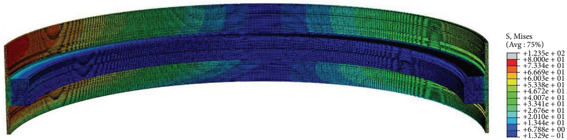
FIGURE 9: Maximum principal stress diagram of flange (unit: MPa).
