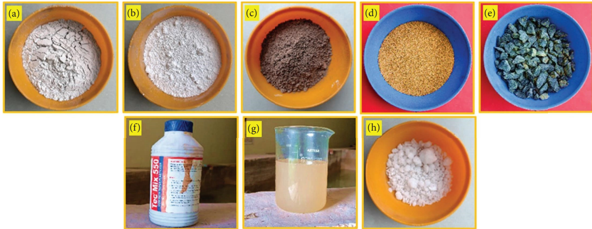
FIGURE 1: Raw materials: (a) silica fume, (b) GGBFS, (c) fly ash, (d) fine aggregate, (e) coarse aggregate, (f) superplasticizer, (g) sodium silicate, and (h) sodium hydroxide.
