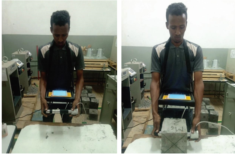
FIGURE 10: UPV calibration and specimen testing.
