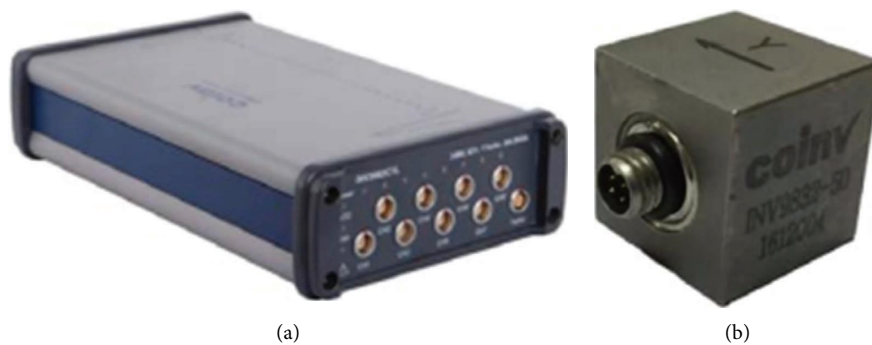
FIGURE 5: Testing equipment: (a) signal acquisition instrument and (b) acceleration transducer.
