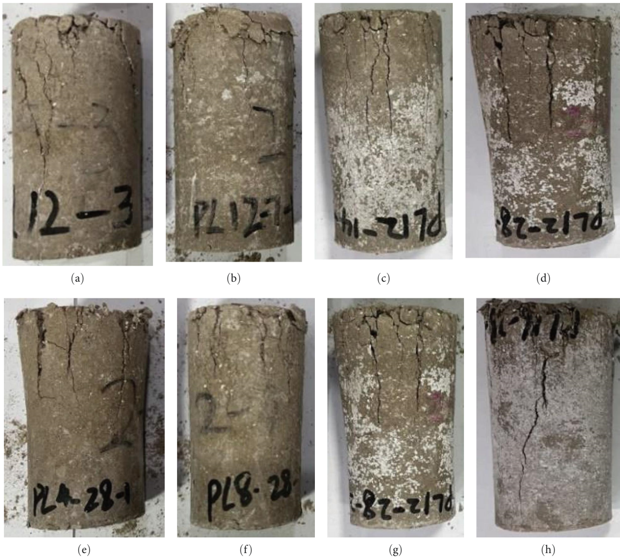
FIGURE 13: Comparison of the failure morphology of the specimen. (a) G12-0, (b) G12-7, (c) G12-14, (d) G12-28, (e) G4-28, (f) G8-28, (g) G12-28, and (h) G16-28.
