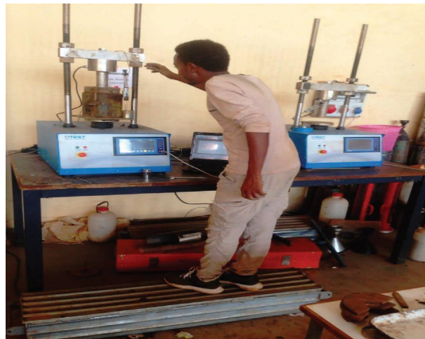
FIGURE 6: Photograph for CBR and unconfined compression test (source: the researchers).
