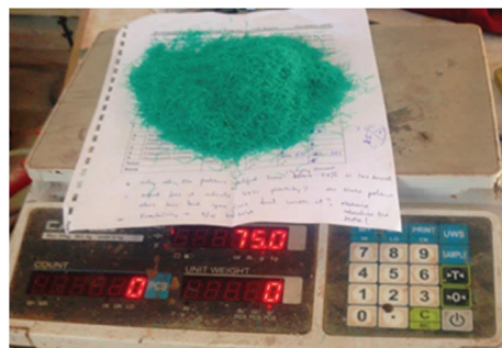
FIGURE 4: Nylon synthetic fiber after trimmed in to 10 and 20 mm lengths (source: the researchers).
