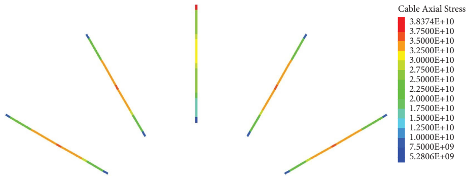
FIGURE 4: Stress distribution of rock bolts in the fully encapsulated rebar bolt supported model.
