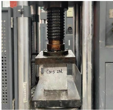
FIGURE 4: Test of concrete cubic compressive strength.
