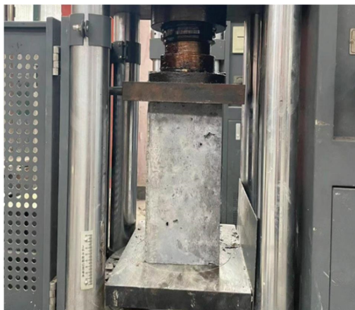
FIGURE 5: Test of concrete uniaxial compressive strength.
