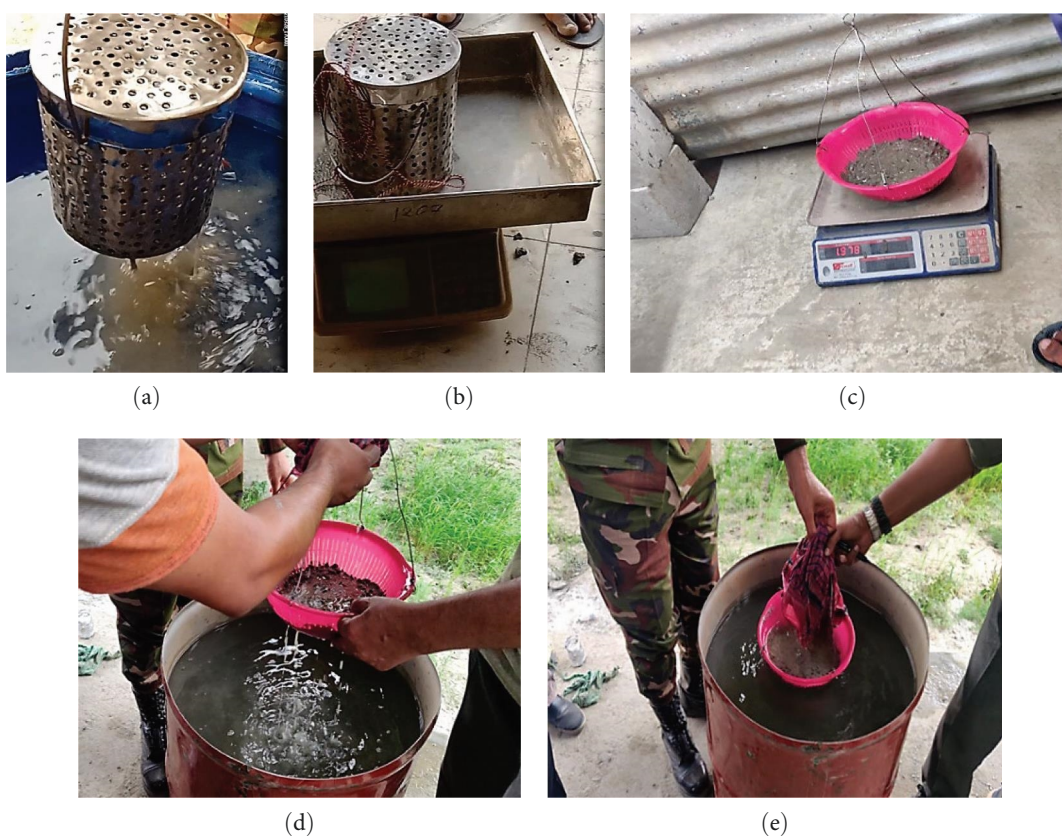
FIGURE 11: (a) and (b) Antidispersal test at laboratory, (c), (d), and (e) at field.
