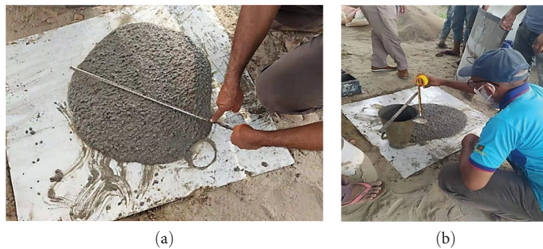
FIGURE 19: (a) and (b) Field slump test of concrete mix.
