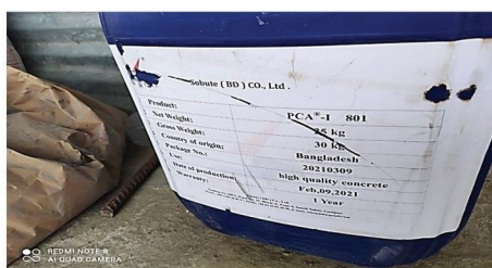
FIGURE 10: Admixture used in the concrete.
