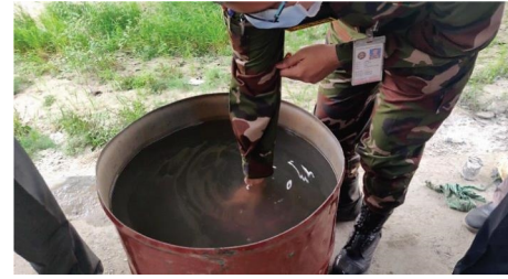
FIGURE 14: Check for pH value after the addition of admixture.
