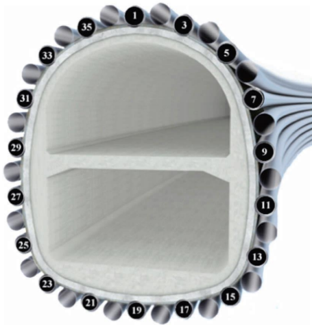
FIGURE 1: Section of Gongbei tunnel.
