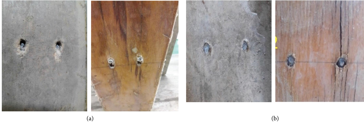
FIGURE 7: Snapped screw remained in the concrete and timber (a) specimen P90h (b) specimen P45h (photo: author).
