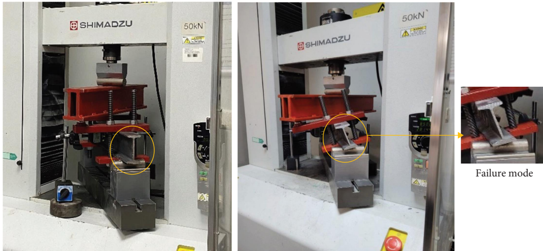
FIGURE 5: The experiment of reference beams under torsion.
