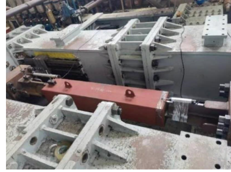
FIGURE 3: Buckling restrained bracings with high ductility.
