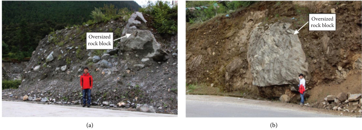
FIGURE 1: S-RM with an oversized rock block (a) in the diluvium and (b) in the moraine.
