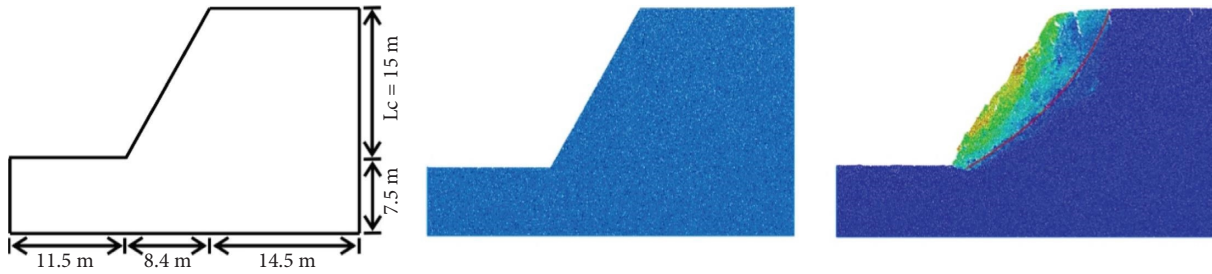
FIGURE 2: The size of the slope model and calculation result of the homogeneous soil slope.
