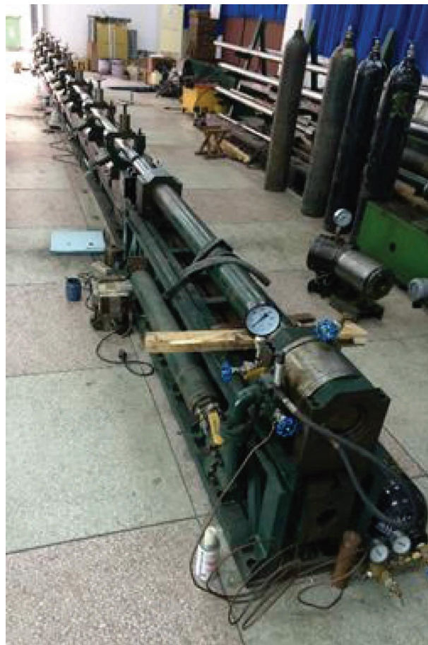
FIGURE 5: Components of the split Hopkinson pressure bar test system.
