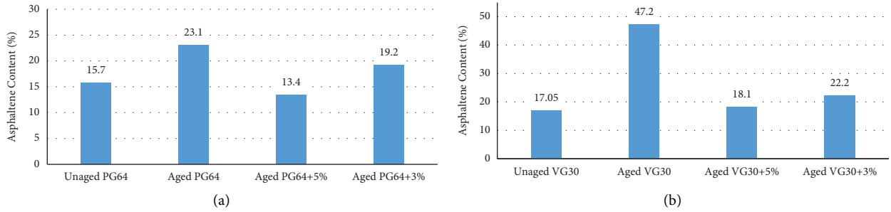
FIGURE 9: Variation in asphaltene content in different bitumens: (a) PG 64-10; (b) VG30.
