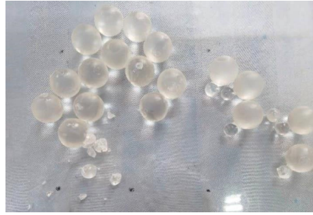
FIGURE 12: Broken PMMA balls.
