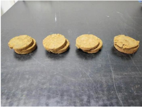
FIGURE 7: Modified expansive soil shear failure specimen.
