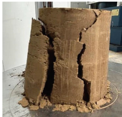
FIGURE 4: Plain expansive soil failure sample.
