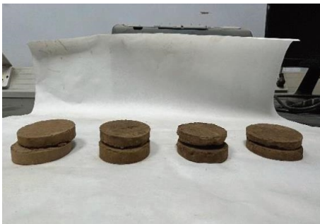
FIGURE 8: Shear failure sample of plain expansive soil.
