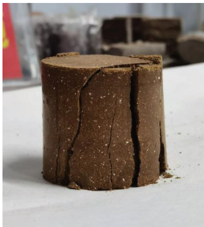
FIGURE 3: Modified expansive soil failure sample.
