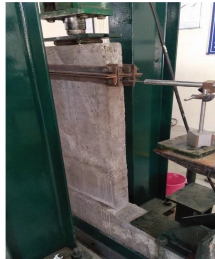
FIGURE 9: Test setup—LVDT arrangement.
