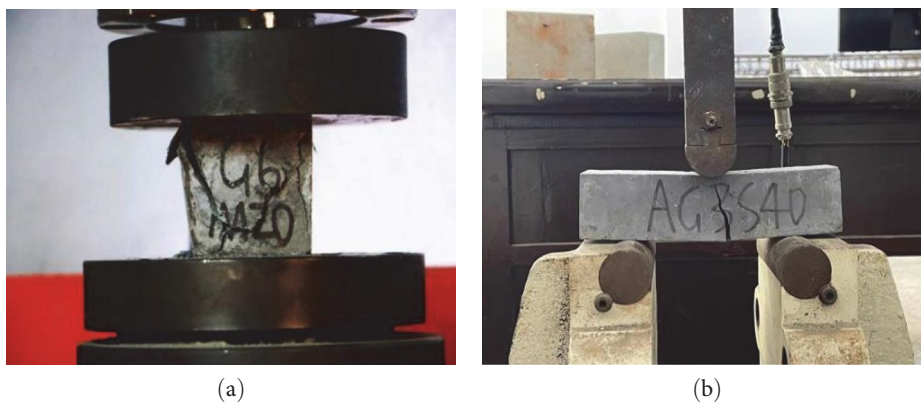
FIGURE 6: Test loading diagram of mechanical properties of solid waste conductive concrete: (a) unconfined compression test and (b) three-point bending test.
