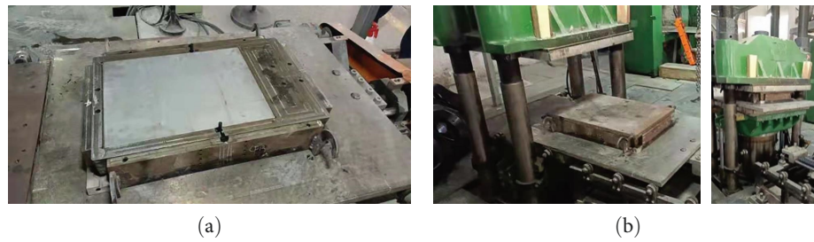
FIGURE 4: Vulcanization process: (a) assembly of the VE layers, steel plates, and mold; (b) flat vulcanizing machine.
