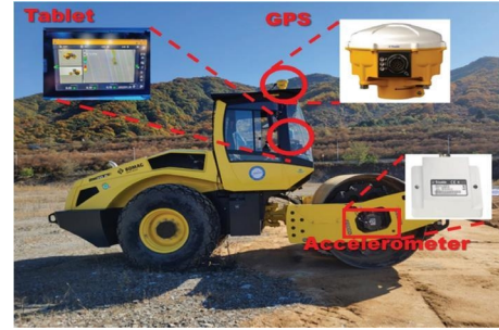
FIGURE 1: An intelligent roller equipped with a tablet, GPS sensor, and accelerometer.
