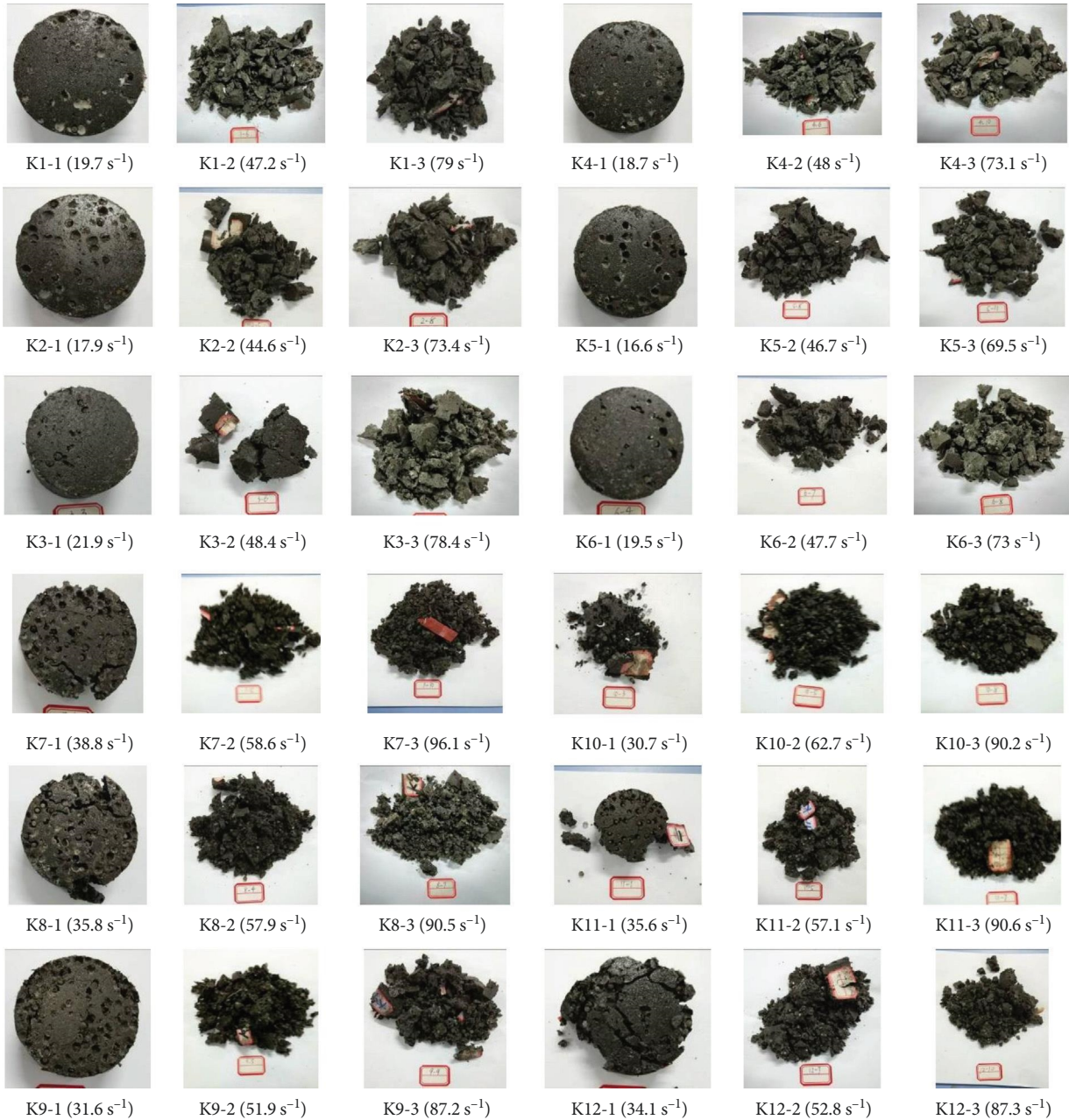
FIGURE 14: Failure of cellular concrete under impact loads.
