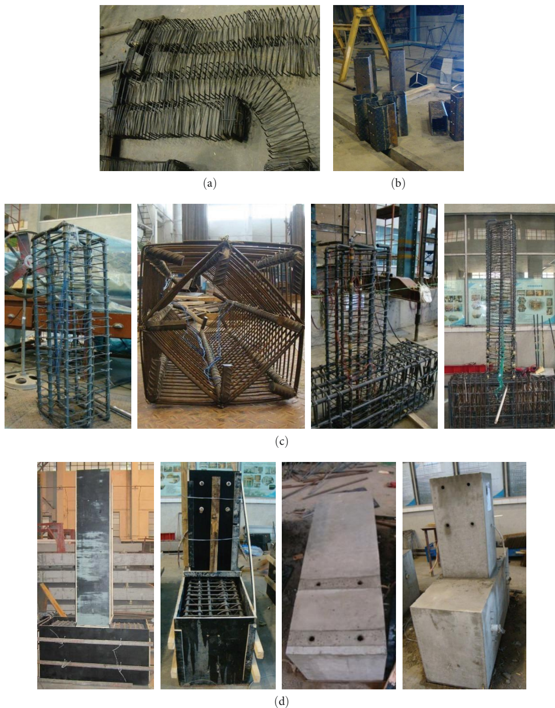
FIGURE 3: Specimen preparation: (a) spiral stirrup; (b) steel plate hoop; (c) reinforcement skeleton; (d) precast concrete.
