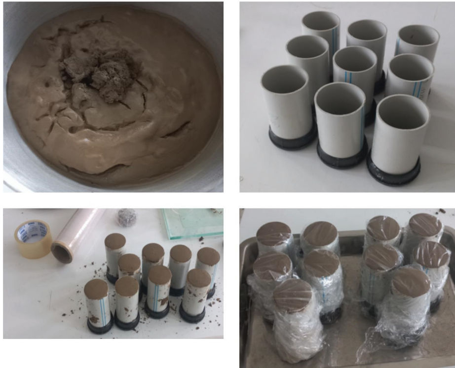
FIGURE 4: UCS specimen preparation using PVC plastic mold.
