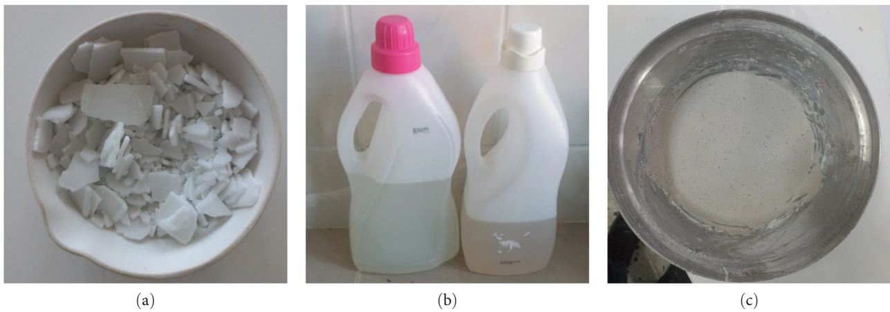
FIGURE 3: Geopolymer slurry preparation using alkali activators: (a) NaOH pellets, (b) NaOH and \text{Na}_2\text{SiO}_3 solutions, and (c) geopolymer slurry.
