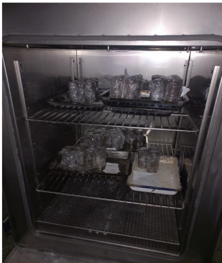
FIGURE 5: Specimens curing chamber.
