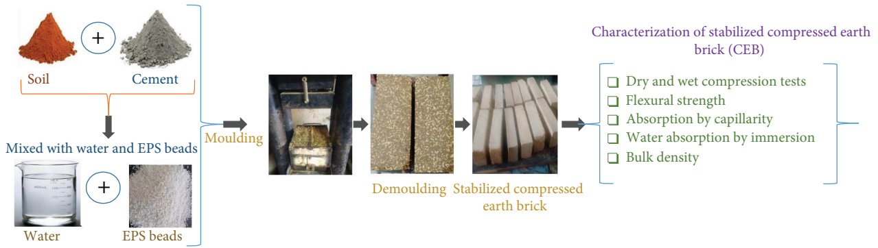
FIGURE 3: Stabilized compressed earth brick (CEB) elaboration process.
