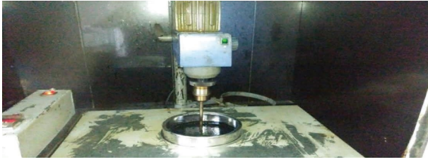
FIGURE 2: The asphalt and additives mixing process.
