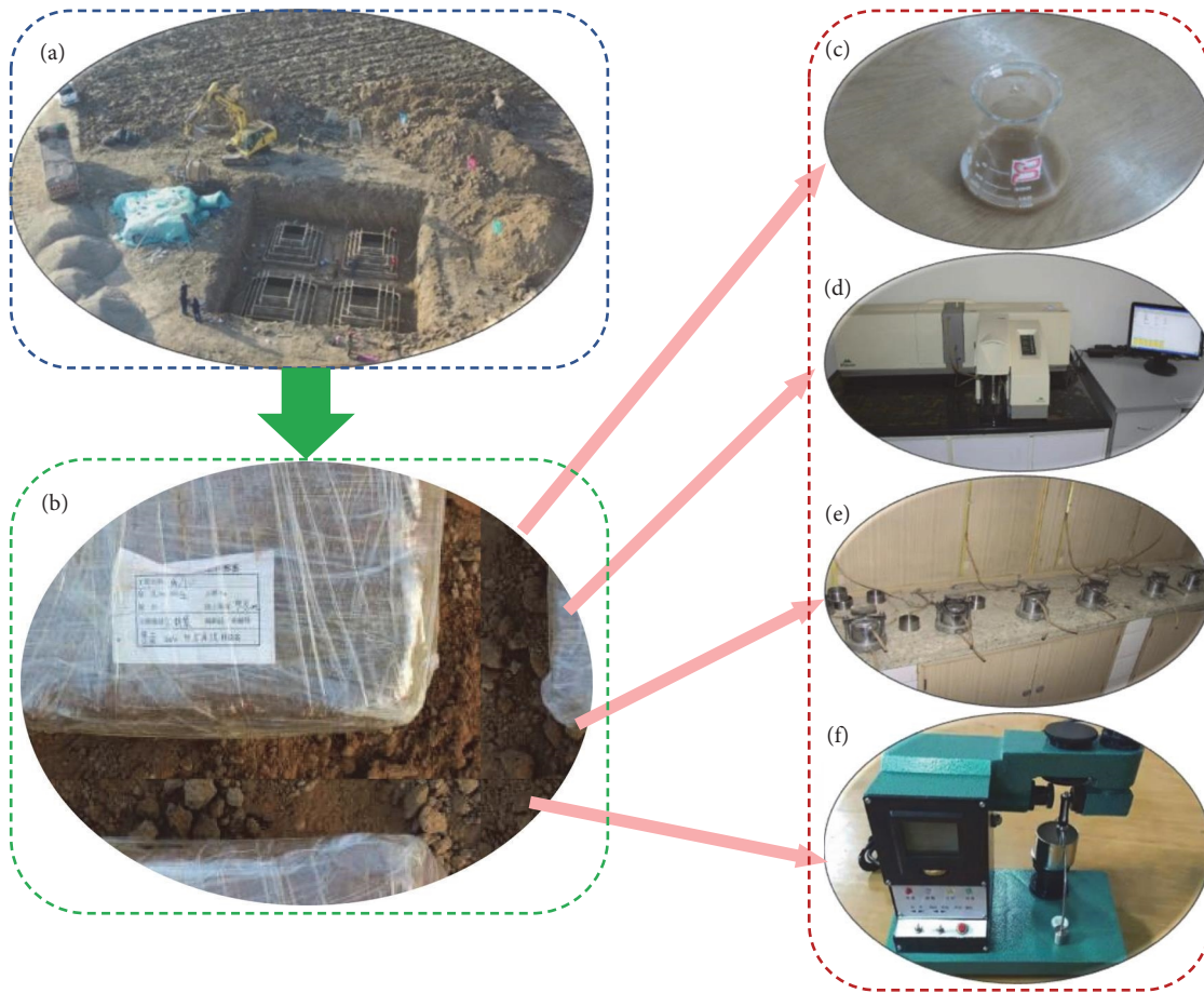
FIGURE 2: Basic physical and mechanical parameters test of loess: (a) iron tower foundation; (b) loess; (c) specific gravity test; (d) particle analysis test; (e) permeability test; (f) liquid plastic limit test.
