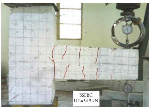
FIGURE 17: Failure pattern of SSFBC specimen.
