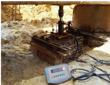
FIGURE 5: Reaction provided by the heaped load.
