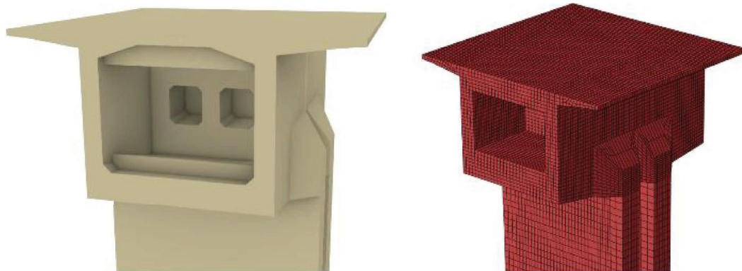
FIGURE 9: The BIM model and finite element model.
