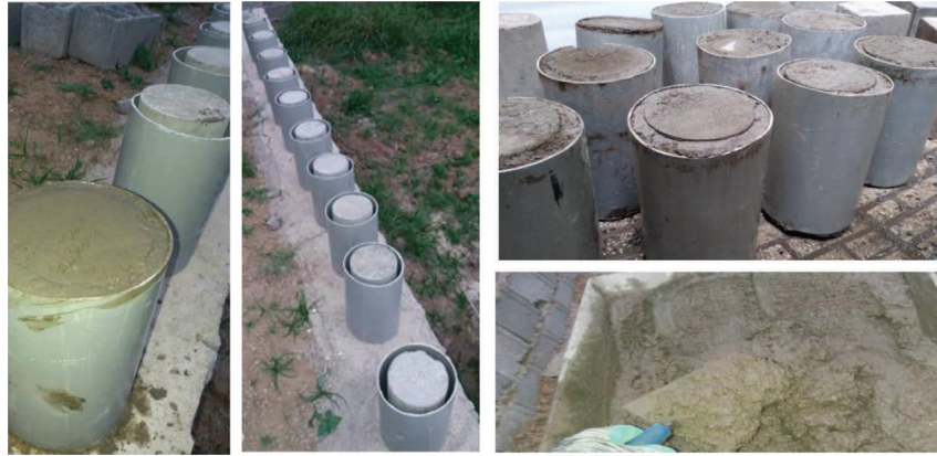
FIGURE 4: Pictures of the manufacturing stages of cylindrical samples.
