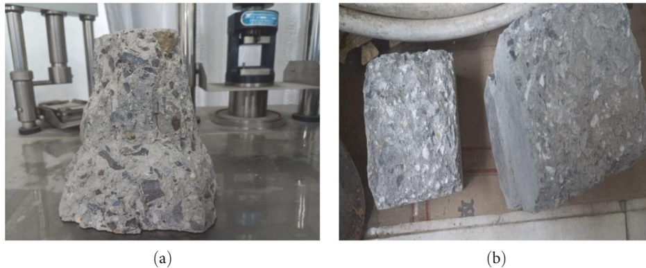
FIGURE 3: Concrete specimens of two different damage states: (a) crushed specimens and (b) chiseled specimens.
