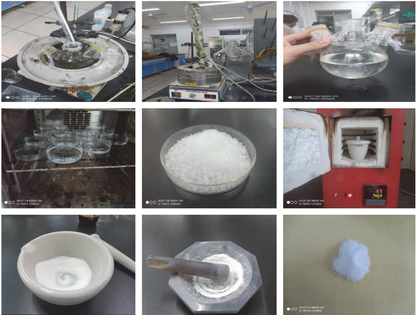
FIGURE 1: The preparation process of CH_3-NS .
