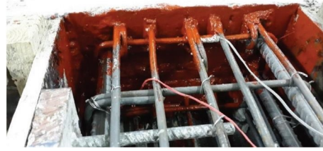
FIGURE 3: Interface between corbel and column painted using adhesive epoxy-based component in specimen M4 ( photo rotated 90° for clarification ).
