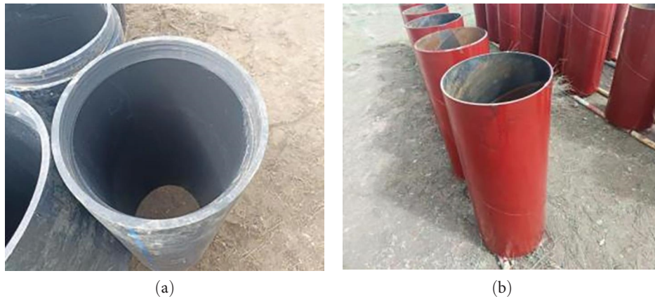
FIGURE 3: Field shield segment: (a) PE tube and (b) steel pipe.
