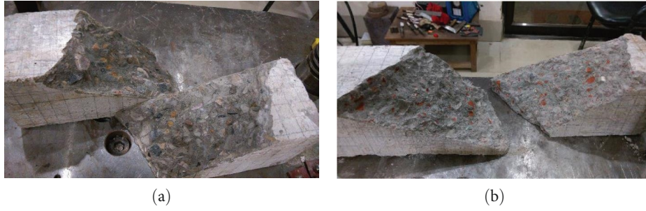
FIGURE 9: Typical crack surface for (a) NSAC and (b) VBAC beams.
