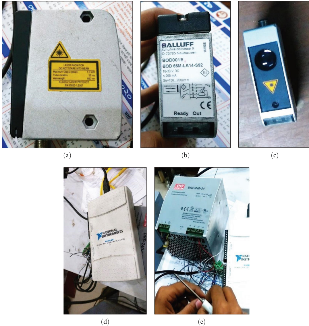
FIGURE 5: (a–c) Side, back, and top view of laser displacement sensor, respectively. (d) data acquisition device and (e) power supply controller of laser displacement sensor.
