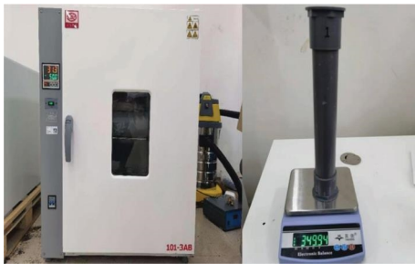
FIGURE 9: Pipe drying and weighing.
