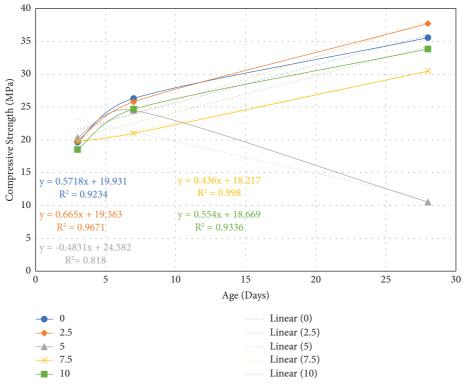
FIGURE 9: Compressive strength of mortar on the effect of age.
