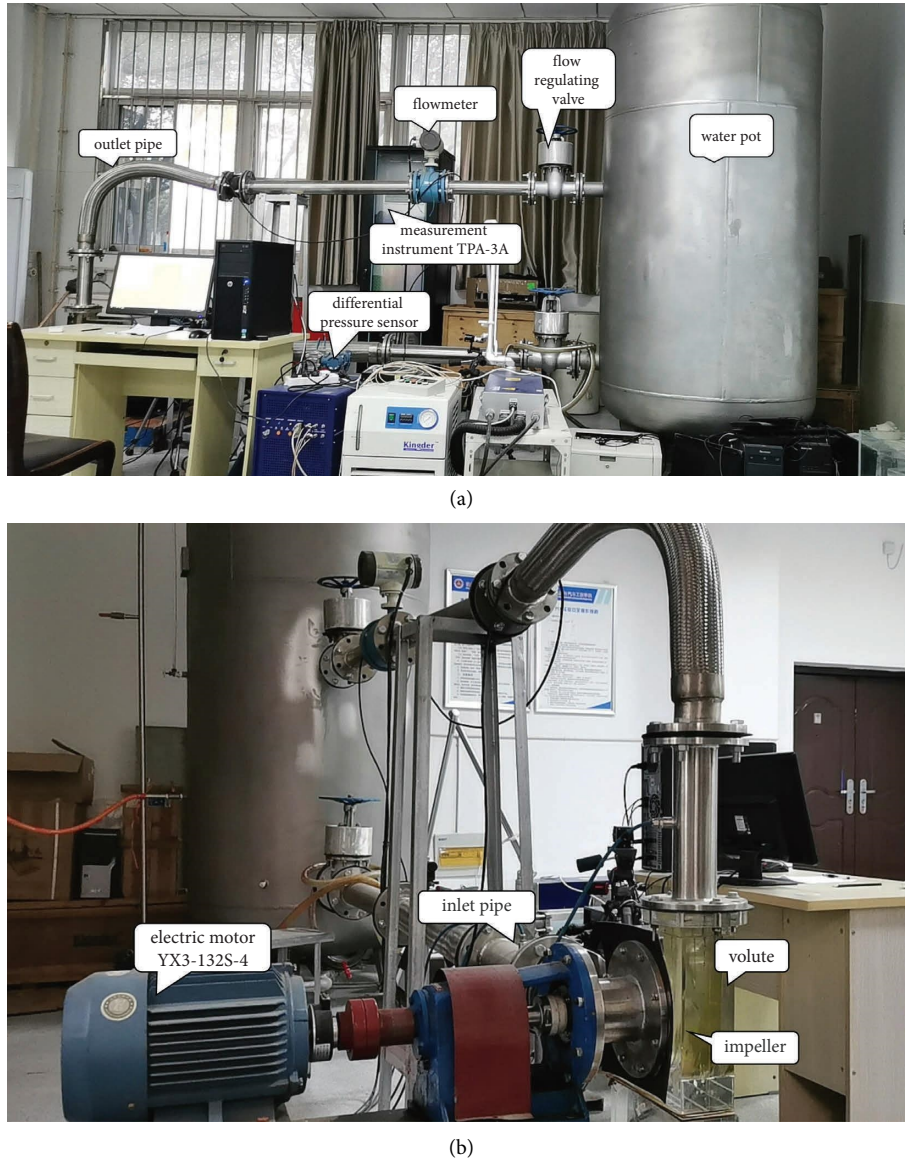
FIGURE 15: Closed pump performance test bench diagram: (a) front view and (b) lateral view.
