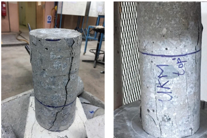
FIGURE 8: Failure of coring SPC and MYC sample after compression.
