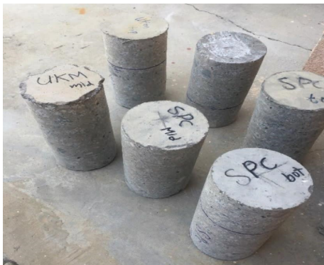
FIGURE 6: Extracted core samples from the tunnel segments.
