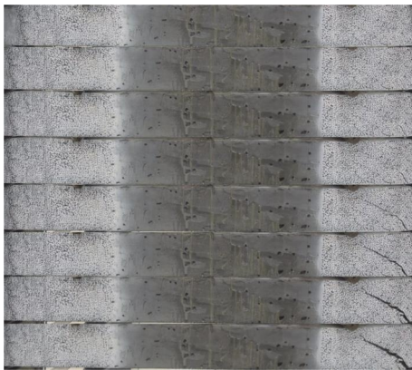
FIGURE 6: Failure mode and crack form of the L30-A1% ASFRPC beam (as an example).
