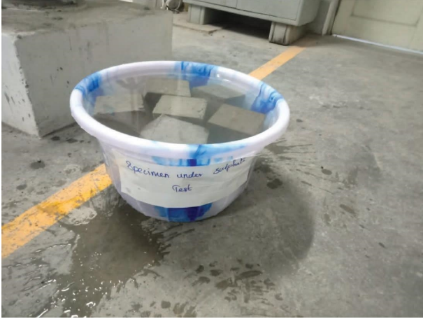
FIGURE 2: Sulphate test setup.
