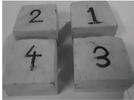
FIGURE 4: Final shape of bricks produced with waste paper [67].
