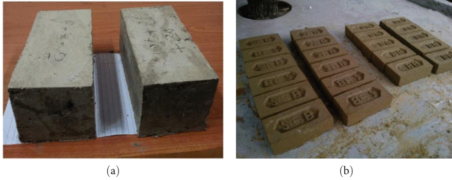
FIGURE 2: (a) Modular bricks using fly ash and lime and (b) nonmodular bricks using paper mill waste [41].
