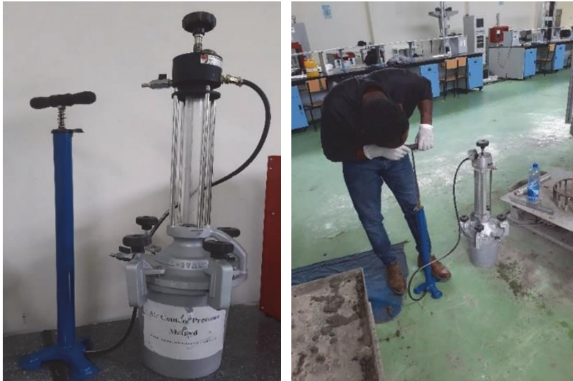
FIGURE 5: Air content (pressure method) testing equipment. Source: Own work, 2022.
