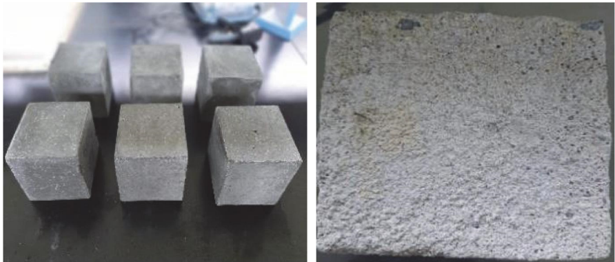
FIGURE 15: Sample concrete specimens color change due to sulfuric acid solution. Source: Own work, 2022.
