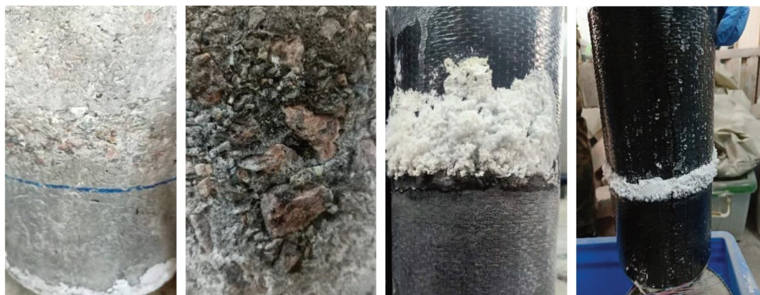
FIGURE 3: Concrete column corroded under continuous half-immersion of sulfate.
