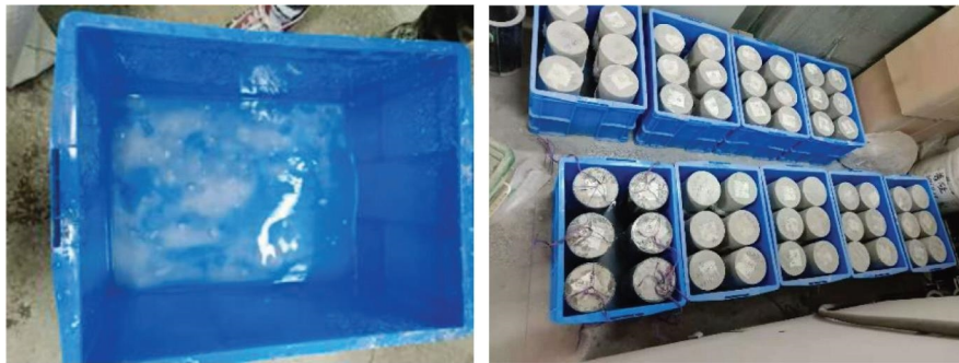
FIGURE 2: Continuous half-immersion test of sulfate.
