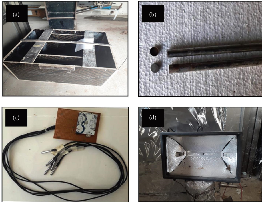
FIGURE 5: PCMs: (a) plywood formwork, (b) PCM steel tubes with caps, (c) thermometers with a data logger, and (d) 1,000 W light.
