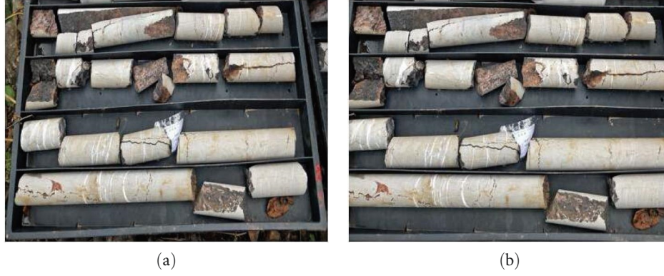
FIGURE 1: Drilling core images before (a) and after (b) the perspective correction.
