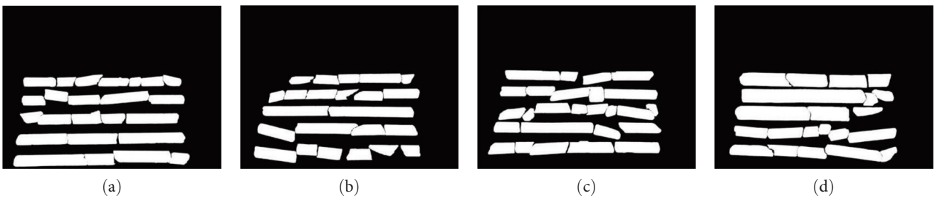
FIGURE 6: Segmentation of drilling core pieces is implemented.
