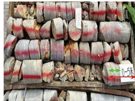
FIGURE 13: The drilling core piece is covered partly by the paper piece, which affects the measurement of the length of the drilling core piece.
