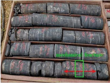
FIGURE 11: The mechanical fractures affect the calculation of the RQD values.
