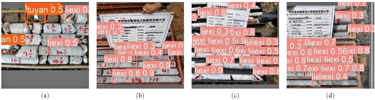
FIGURE 10: Lengths of the drilling core pieces are measured automatically.
