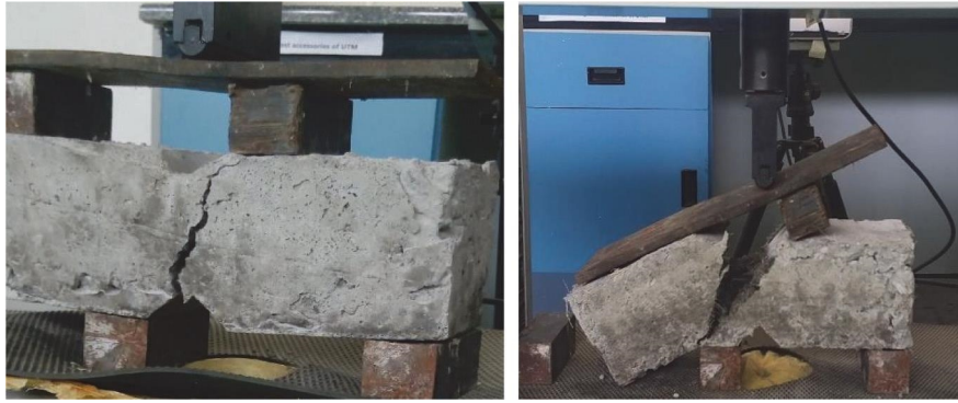
FIGURE 15: Shear failure mode and cracking pattern.
