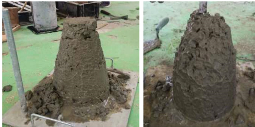
FIGURE 4: Slump test (workability).
