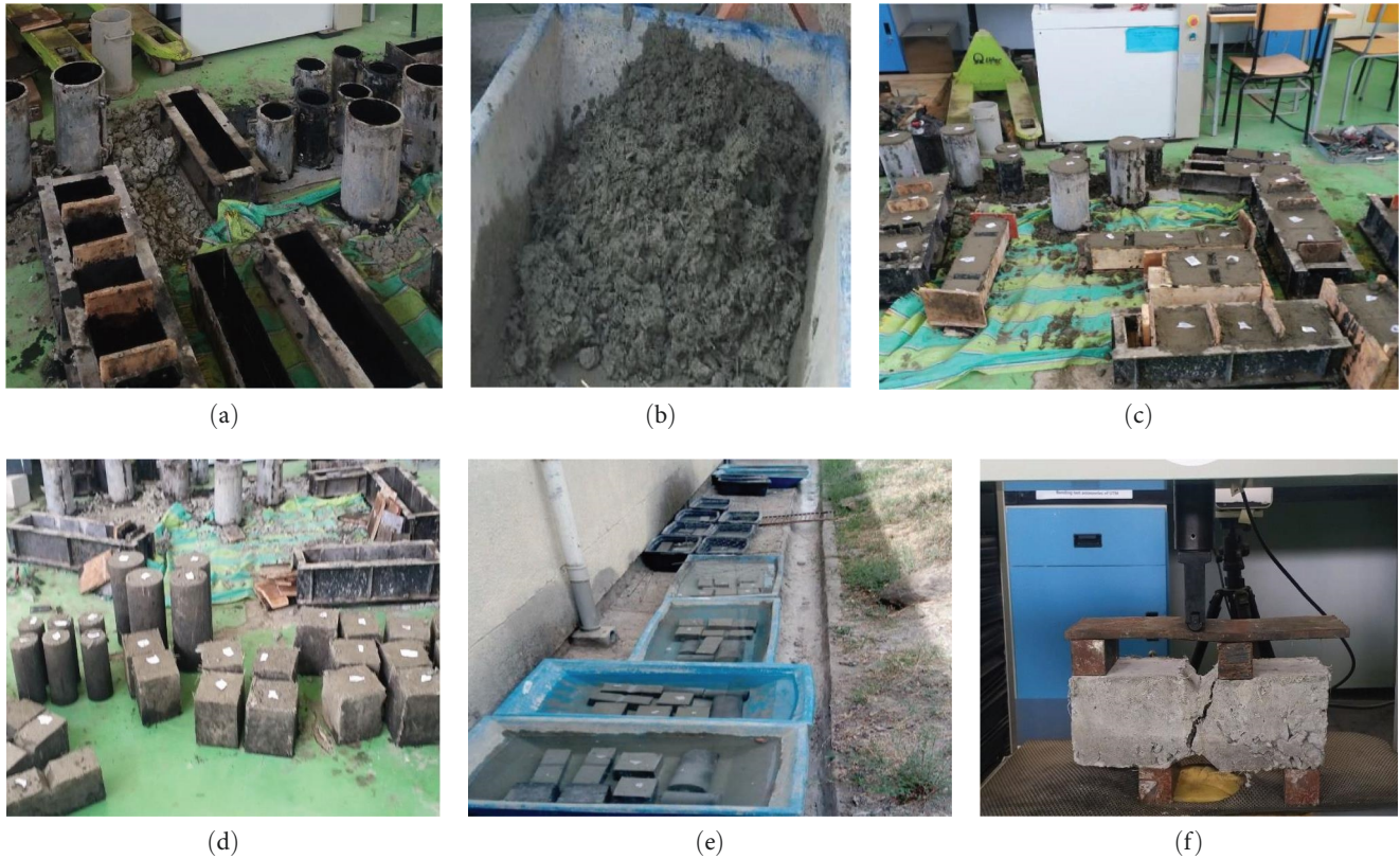
FIGURE 3: (a) Formwork oiling, (b) mixing, (c) molding, (d) formwork removing, (e) curing, and (f) testing.
